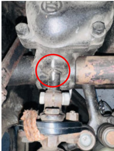
Input alignment shaft of ZF steering box
