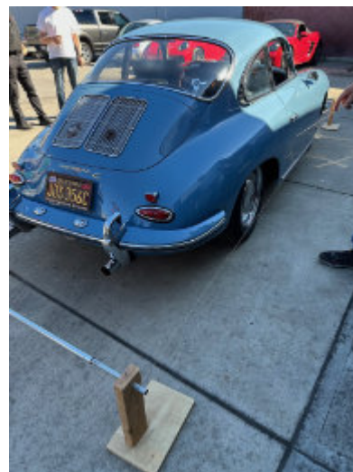
String box stands. Strings are 68" apart and 13" from the floor.
