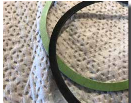
Two Oil Filter Gaskets, One Rubber and One Paper
