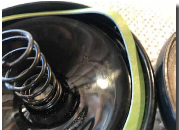
Fram Oil Filter paper Gasket not Fitting Cover
