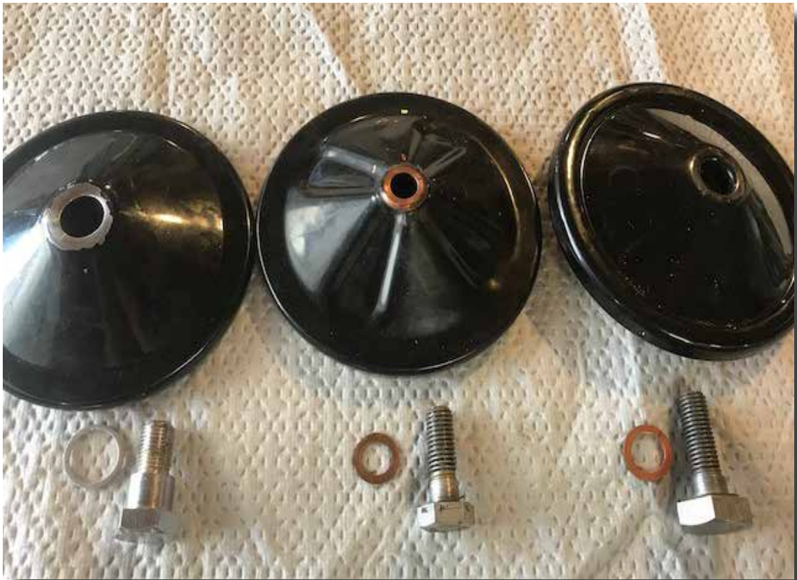
Three different Oil Filter Covers, Bolts and Crushable Washers
