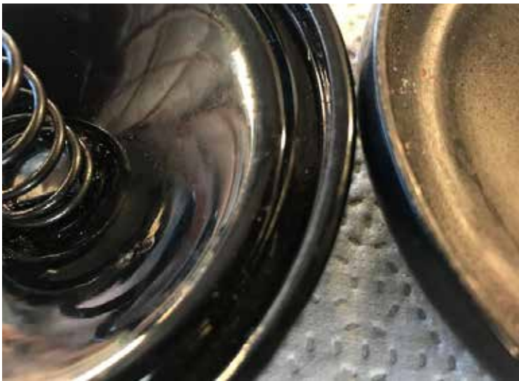
Inside Oil Filter Cover Lips, Fram left, H-Filter Right
